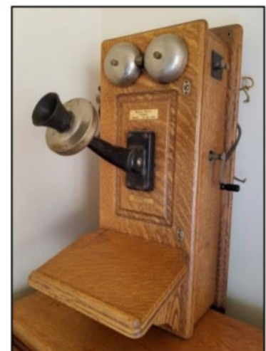
Actual Guglielmetti party-line telephone shows mouthpiece, hand crank, and bells. The receiver hangs on the left side. Photo courtesy of Alfred Guglielmetti.
